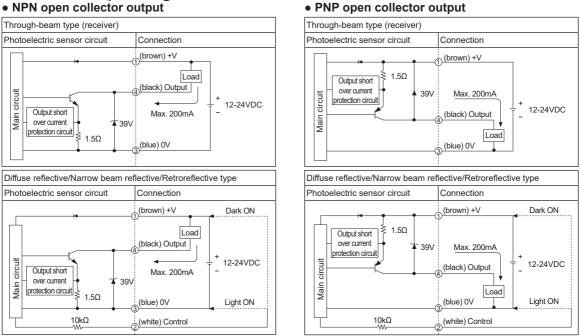
\*Before using this unit, select Light ON/Dark ON with control wire. (light on: connect control wire 0V / dark on: connect control wire with +V) \*Control wire is only for Diffuse reflective/Narrow beam reflective/Retroreflective type.
