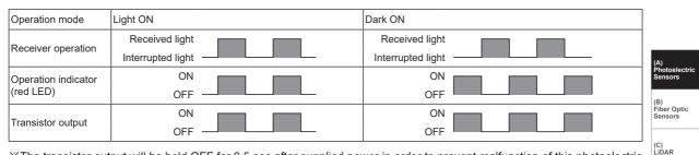
\* The transistor output will be held OFF for 0.5 sec after supplied power in order to prevent malfunction of this photoelectric sensor (except through-beam type).
