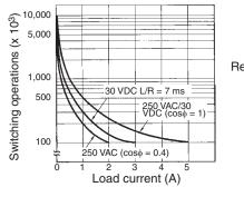
Reference: A maximum current of 0.15 A can be switched at 125 VDC ( $\cos\phi = 1$ ) and a maximum current of 0.1A can be switched at 125V DC and L/R = 7ms. In both cases, a life of 100,000 operations can be expected. The minimum applicable load is 10 mA at 5 VDC (failure level: P).
