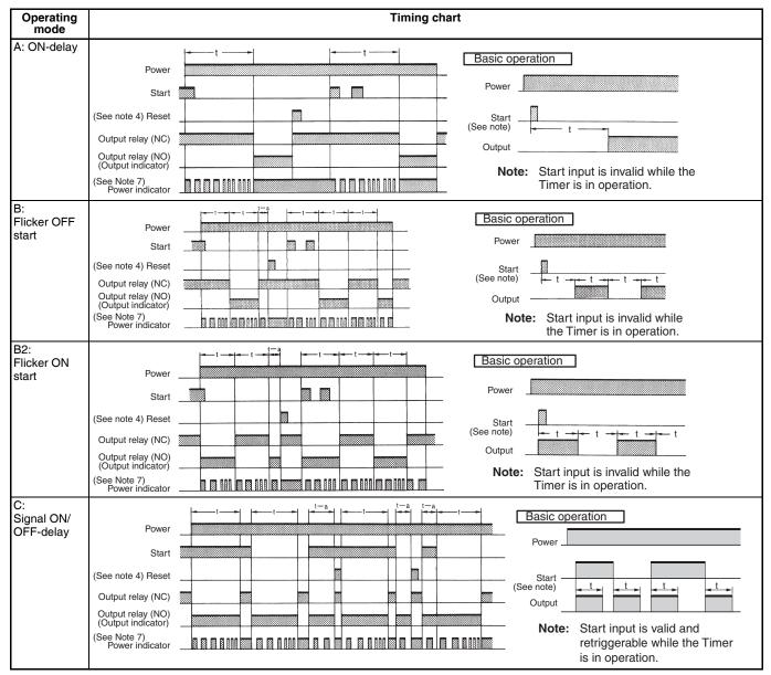
Note: 1. Allow at least 0.1 s for the Timer reset time if the power supply is reset due to an interruption in the power supply.
