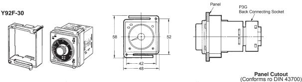
**Note1:** The adapters for two or more timers mounted in a vertical line are different in orientation from those mounted in a horizontal line.
