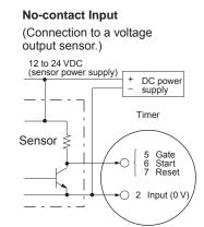
Operates with transistor ON
