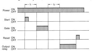
Note: 1. Allow at least 0.1 s for the Timer reset time if the power supply is reset due to an interruption in the power supply.
