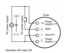
**Note:** Refer to the signal levels in the following table and be aware of the minimum applicable load of the relay.
