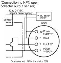
**Note:** The input circuit is isolated from the power supply circuit. Thus, an NPN transistor can be connected.
