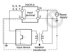
The H3CR-A's power supply terminal 2 is a common terminal for input signals to the Timer. Do not disconnect the wires on terminal 2, otherwise the internal circuitry of the Timer will be damaged.
