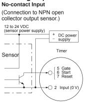
Timer 5 Gate 6 Start 7 Reset 0 2 Input (0 V) Operates with relay ON
