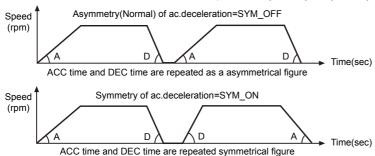
XIt is able to set the gradient(acceleration and deceleration time) as ACC/DEC time.
