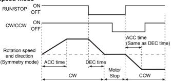
It accelerates up to RUN speed during ACC time after RUN signal is ON and decelerates during DEC time after it is OFF. It is disable to change the direction during the signal is ON and it takes 0.5sec. for deceleration when DEC time is "0%".
