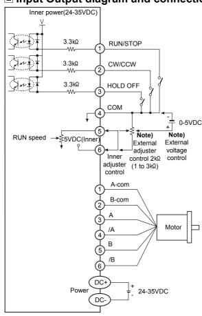
Note) Inner adjuster is correlated to external adjuster control and external voltage control. Make sure that inner adjuster must be set to maximum in order to set maximum RUN speed using external adjuster and external voltage.
