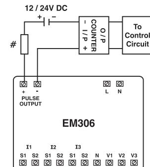
Pulse output from meter can be used as alarm generator or total energy controller by interfacing it with Pre settable counter and control circuits (Contactors, Relay, Trip Circuit).
