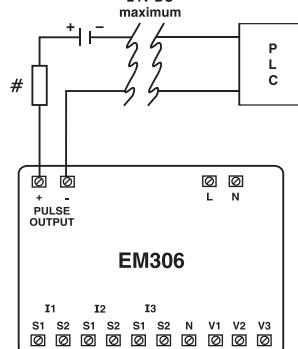
Pulse output from meter can be interfaced into a process through a PLC for on line control of energy content in the process.
