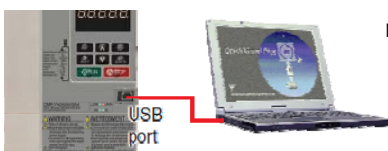
● Connecting L1000 and a PC with USB
