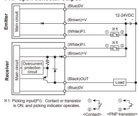
\*\*Picking indicator: When external picking input(P.I) is short-circuited with OUT(Black), it is operated same as ON/OFF status of control output.
