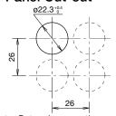
Note: Determine mounting centers to ensure operation.
