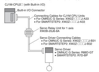
When two axes are used, two Connecting Cables are required at the Servo Driver for each Servo Relay Unit.
