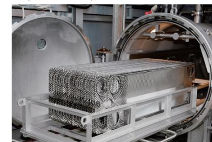
High Temperature and High Pressure Cleaning Device
