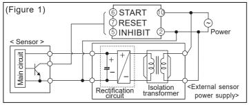
• In order to avoid leakage current flowing, connect resistance and condenser as (Figure 2). If connect as (Figure 1), it may cause malfunction due to leakage current.
