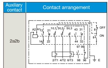
Note 1) The above figure gives an example of when the main circuit and operating circuit use the same power supply. The solid line is already wired. The dashed line and two-dot chain line sections must be wired. (Use the wires enclosed with the unit to wire the two-dot chain line sections.)
