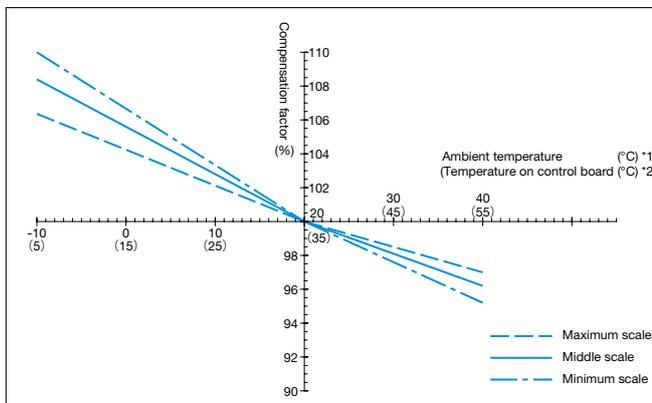
Diagram 1. Ambient temperature compensation curve (T18 frame)
