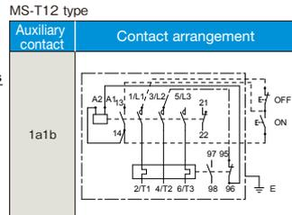
Note 1) The above figure gives an example of when the main circuit and operating circuit use the same power supply. The solid line is already wired. The dashed line and two-dot chain line sections must be wired. (Use the wires enclosed with the unit to wire the two-dot chain line sections.)
