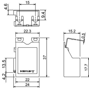
The outline dimensions of the magnetic contactor and magnetic relay do not differ after mounting.
