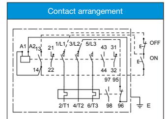
Note 1) The above figure gives an example of when the main circuit and operating circuit use the same power supply. The solid line is already wired. The dashed line and two-dot chain line sections must be wired. (Use the wires enclosed with the unit to wire the two-dot chain line sections.)
