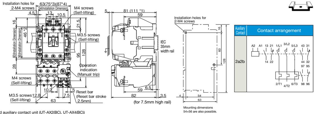
\*1 dimensions: With head mounted auxiliary contact unit (UT-AX2(BC), UT-AX4(BC))
