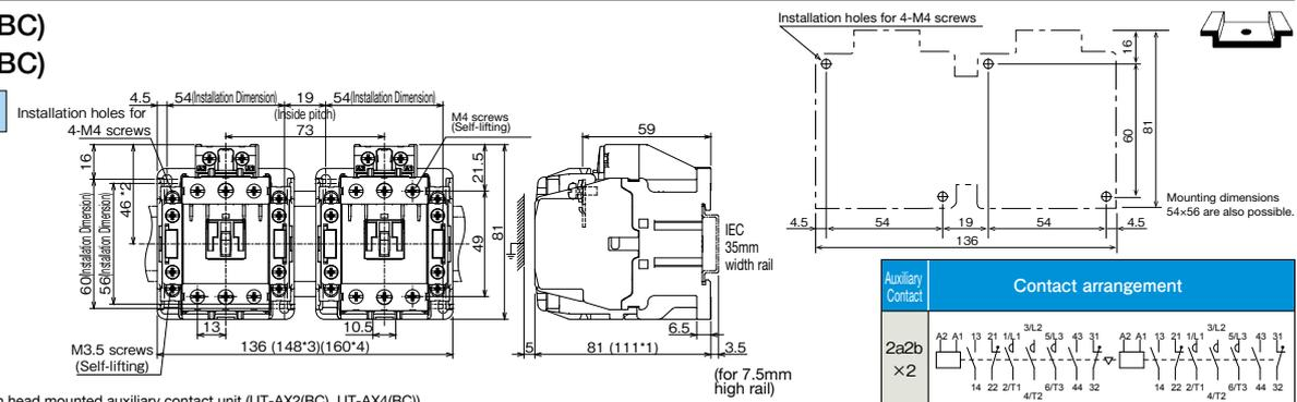
\*1 dimensions: With head mounted auxiliary contact unit (UT-AX2(BC), UT-AX4(BC))
