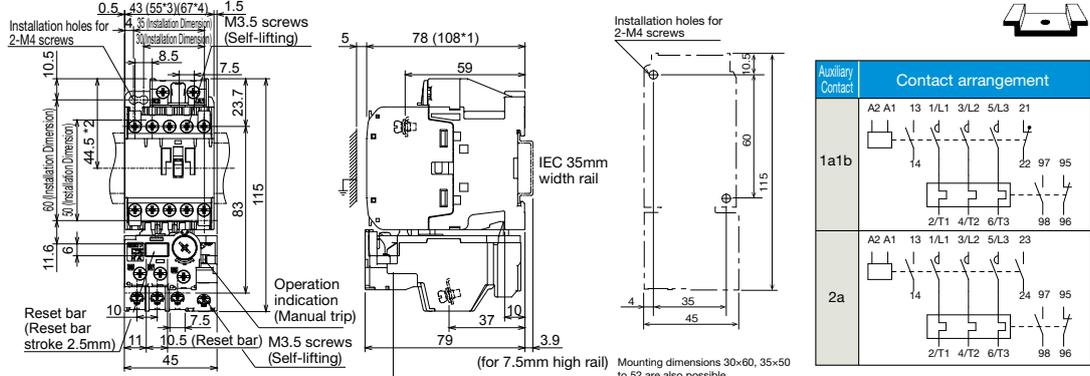
\*1 dimensions: With head mounted auxiliary contact unit (UT-AX2(BC), UT-AX4(BC))
