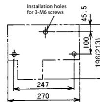
Note: Values in parentheses apply for MSO-2XN80 heater nominal 67A and MSO-2XN95 heater nominal 67A or 82A.
