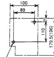
Note: Values in parentheses apply for MSO-N80 heater nominal 67A and MSO-N95 heater nominal 67A or 82A.
