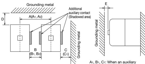
A<sub>1</sub>, B<sub>1</sub>, C<sub>1</sub>: When an auxiliary contact is added to the shadowed area
