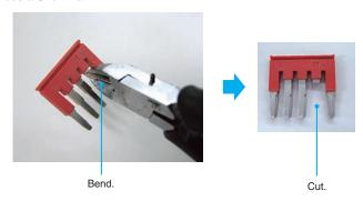
If a Short Bar that has the required pins is not available, you can combine more than one Short Bar to short the required Terminal Blocks.
