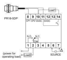
• The sum of operating current capacity of load 1 and sensor should not be over external power capacity (50mA).
