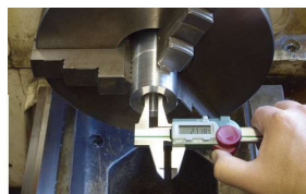
Allows easy measurement of I/D during turning operation
