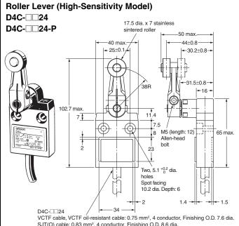
SJT(O) cable: 0.83 mm2, 4 conductor, Finishing O.D. 8.6 dia.
