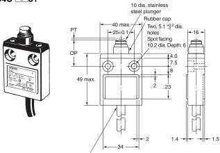
VCTF cable, VCTF oil-resistant cable: 0.75 mm², 4 conductor, Finishing O.D. 7.6 dia. SJT(O) cable: 0.83 mm², 4 conductor, Finishing O.D. 8.6 dia.
