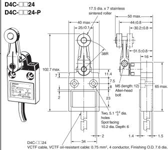
SJT(O) cable: 0.83 mm2, 4 conductor, Finishing O.D. 8.6 dia.
