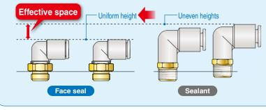
Allows for neat and compact piping without protruding threads <Application example>
