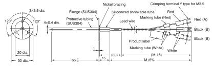
Note: The protective tubing is of pipe construction, which must not be bent.
