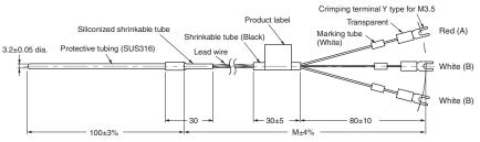
Note: 1. The protective tubing is of pipe construction, which must not be bent.
