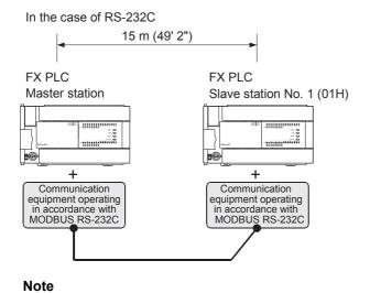
MODBUS Slave Nodes do not need to be numbered in any specific order.
