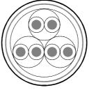
Example of three-pair cable structural drawing
