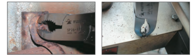
For rusty screw For stripped screw
