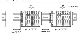
To mount the Power Supply to a DIN Rail, hook portion (A) of the Power Supply onto the DIN Rail and press the Power Supply in direction (B) until you hear it lock into place. Make sure that the catch on the Mounting Bracket is engaged with the DIN Rail.
