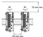
The above figure shows a model with the terminal block facing forward.
