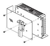
Accessories (4 locations) Be sure to use the accessory screws. Mounting screw tightening torque: 0.48 to 0.59 N·m for M3 screws
