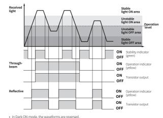
Operation indicator and transistor output differ from the sensing method
