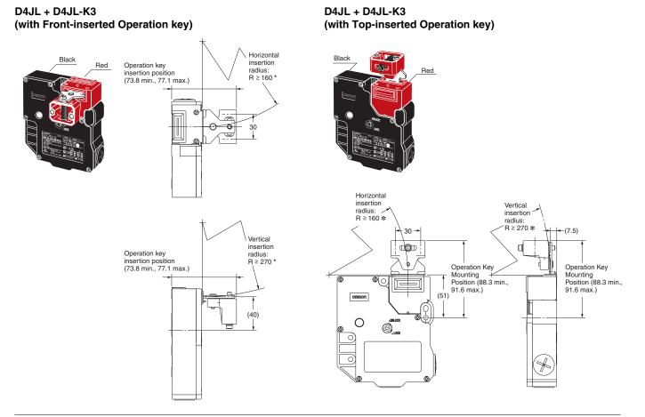
\* Insertion radii apply when the rotational center of the Operation Key is in line with a line extending from the front or top Head surface.
