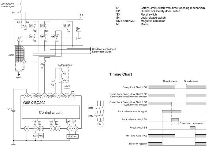
Note: The lock release enable signal must be configured so that it should turn ON after dangerous movement is stopped and safety is ensured for the door to open.
