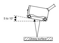
• If there is a reflective surface beneath the sensor, the reflected light may reflect off the surface of the reflective object. Make sure that the sensor is tilted upwards as shown in the figure, or install the sensor distant to the reflective surface.
