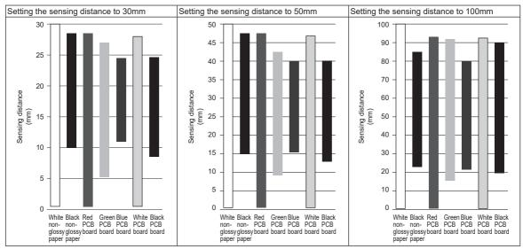
※ Above graphs are rated for each sensing target at the status that the sensing target is the white non-glossy paper and the sensing distance is set to 30mm, 50mm, 100mm.
