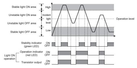
% The waveforms of 'Operation indicator' and 'Transistor output' are for Light ON operation. The waveforms are reversed for Dark ON operation.
