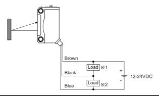
%1: Load connection of NPN open collector output%2: Load connection of PNP open collector output
