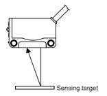
• If the sensing target has a glossy surface, mount the sensor at a 5 to 10° angle as shown in the figure. Check to see that there is no influence from background objects.
