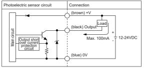
• PNP open collector output Photoelectric sensor circuit Connection (brown) +V (brown) +V (brown) +V (black) Output (black) Output (blue) 0V (blue
