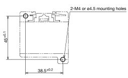
Recommended tightening torque: 0.6 - 0.9 N·m
