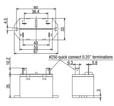
RL2B-T Quick Connect Terminal 2 Pole Flange Mount
