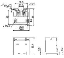
RL2N-D Screw Terminal 2 Pole DIN Rail Mount
