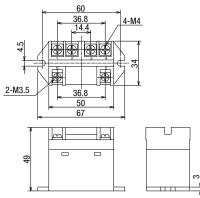
Recommended tightening torque: Coil terminals (M3.5): 0.7 - 0.9 N·m, Contact terminals (M4): 1.0 - 1.4 N·m
