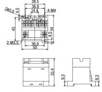
Recommended tightening torque: Coil terminals (M3.5): 0.7 - 0.9 N·m, Contact terminals (M4): 1.0 - 1.4 N·m
