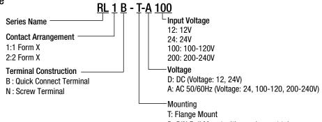
D: DIN Rail Mount with panel mount tabs
