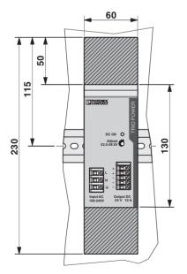
Mounting position: Installation depth 152.5 mm (+ DIN rail)
