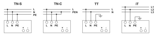
The connection for 100 V AC ... 240 V AC is made using the L, N and PE screw connections. The device can be connected to 1-phase AC networks or to two of the phase conductors of 3-phase networks (TN, TT or IT networks in acc. with VDE 0100-300/IEC 60364-3) with nominal voltages of 100 V AC ... 240 V AC. In the case of input voltages > 300 V AC, the device switches off for its own safety. After the overvoltage has ceased, the device starts automatically within a few seconds.
