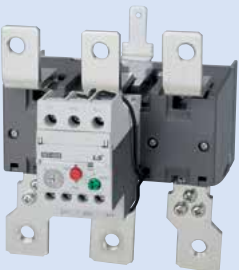
MT-400 Overload relay directly mountable to the contactor Current range 85-400A
