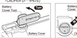
③ Insert the new battery with the  $\oplus$  side outward.
