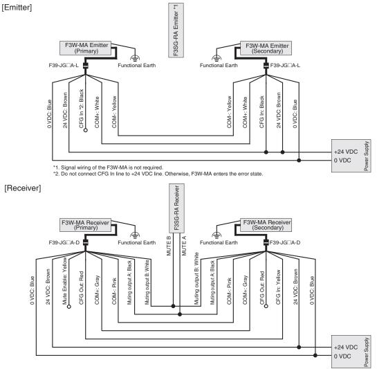
Note: The wiring examples in later pages do not indicate functional earth. To use functional earth, wire an earth cable according to the example above. Refer to Smart Muting Actuator F3W-MA Series User's Manual for more information.
