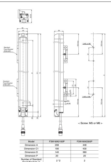
\*1. The number of brackets required to mount either one of emitter and receiver.
