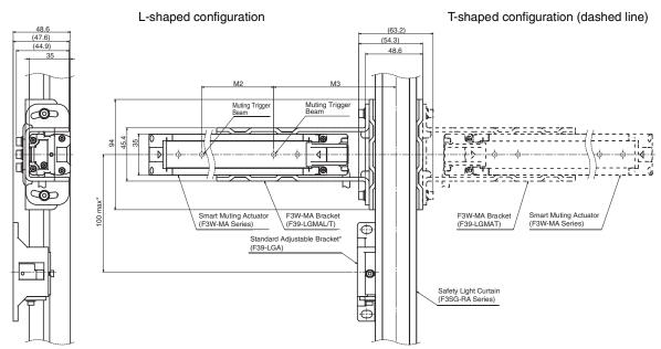
**Note:** When mounting an F3W-MA0300P in the L-shaped configuration, the shock resistance becomes as follows. Shock resistance: 50 m/s<sup>2</sup>, 1000 shocks for all 3 axes
