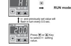
XLow value setting range : Min. display pressure ≤ L □ ≤ Max. display pressure ※High value setting range : L □ ≤ HI < Max. display pressure</p>
