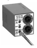
Use a flat screwdriver with a diameter of 4 mm maximum to turn Time Range Selector and gain time range as shown in the table below. Note that the selectors do not turn infinitely.
