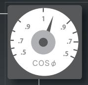
Depending on the terms of the contract, electricity fees may be determined by the power factor. Phase advancing capacitors are used to improve the power factor. Three-phase imbalance, however, may diminish their effect, leading to higher electricity fees.
