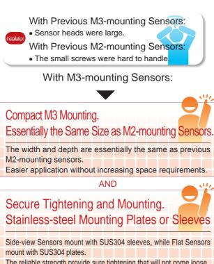
The reliable strength provide sure tightening that will not come loose. Damage from overtightening is also prevented for sure mounting.
