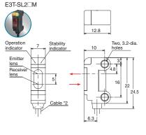
\*1. The dotted line indicates the Receiver. \*2. 4-dia. vinyl-insulated round cable with 2 or 3 conductors (Conductor cross section: 0.1 mm<sup>2</sup> (AWG27),Insulator diameter: 0.7 mm), Standard length: 2 m
