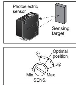
※ The sensing distance indicated on specification chart is against 100 X 100mm of non-glossy white paper. Be sure that it can be different by size, surface and gloss of target.
