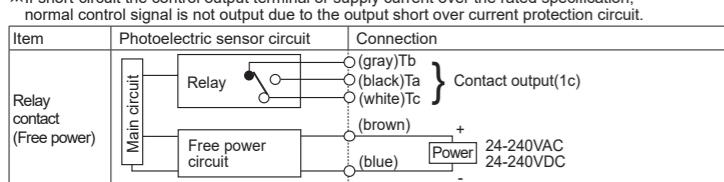
※ Non-using wires must be insulated.
