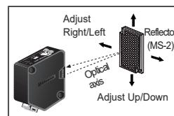
※ If use more than 2 photoelectric sensors in parallel, the space between them should be more than 30cm.
