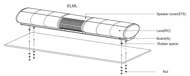
• First, machine taps or holes on the mounting surface .
