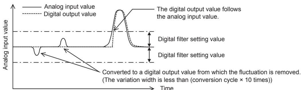
Digital filter requires the A/D conversion values for 23 times to remove the fluctuation which is smaller than the digital filter setting value. Therefore, when using the digital filter, the first digital output value is updated at the timing when the A/D conversion values for 23 times are completed.
