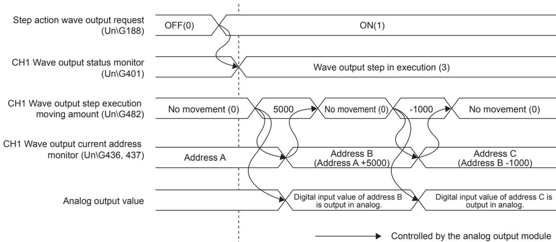
By turning 'Step action wave output request' (UnG188) OFF (0) → ON (1), change the status to Wave output step execution in progress. By setting the value in 'CH1 Wave output step action movement amount' (UnG482) during wave output step execution, control moves to the address of the wave data to be subjected to the output test. For the value in 'CH1 Wave output step action movement amount' (UnG482), set the amount by which to move it from the address of the current wave data.
