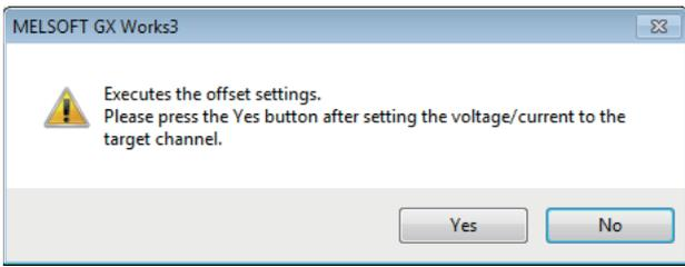
6. Input the offset value voltage "0 V" to the terminal of the target channel (CH1) and click the [Yes] button.
