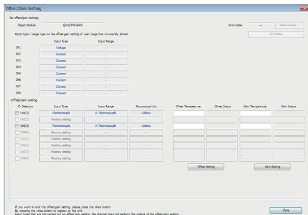
4. Mark the checkbox of the channel (CH1) where offset and gain values are to be set.
