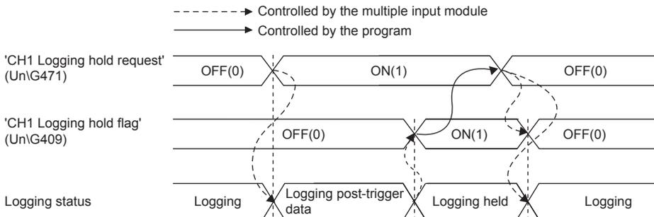
Logging does not stop when 'CH1 Logging hold request' (Un\G471) is changed from on → off before ON (1) is stored in 'CH1 Logging hold flag' (Un\G409).
