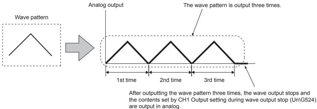
For the analog output module, "repetitive control" that outputs the same wave pattern repeatedly is defined as follows.
