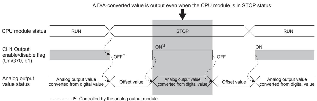
\*1 When the CPU module status changes to STOP, 'CH1 Output enable/disable flag' (Un\G70, b1) turns off.
