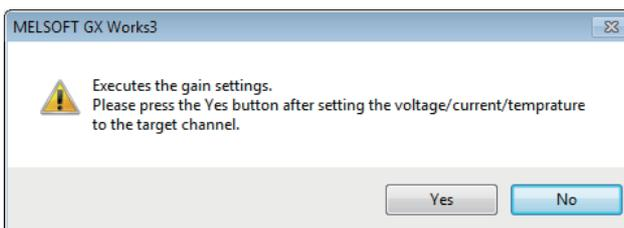
11. Input the gain value temperature "100°C" to the terminal of the target channel (CH1) and click the [Yes] button.
