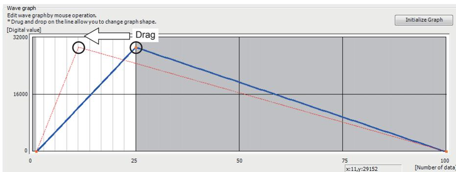
The end point position can be adjusted also by changing the "End point" and "Digital value" values in "Wave detail setting".
