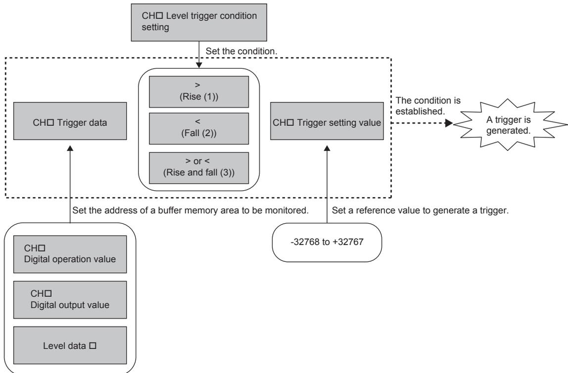
For example if trying to generate a hold trigger when a value in 'CH1 Digital output value' (Un\G400) is greater than 1000, set as follows.
