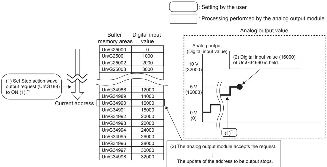
\*1 The contents described here is the case when the wave output status is the wave output in progress at the timing of (1). If the status is other than the wave output in progress, the following value is output at the timing of (2).
