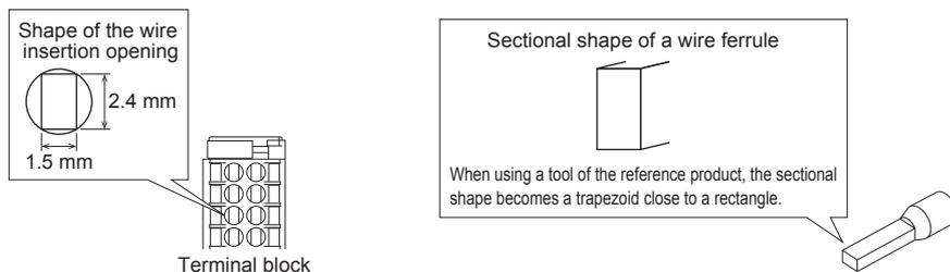
The following table shows wire ferrules and its associated tools compatible with the terminal block. The shape of the wire ferrule differs depending on the crimp tool to be used, use the reference product. If the product other than referenced products is used, the wire ferrule cannot be removed. Sufficiently confirm that the wire ferrule can be removed before use.
