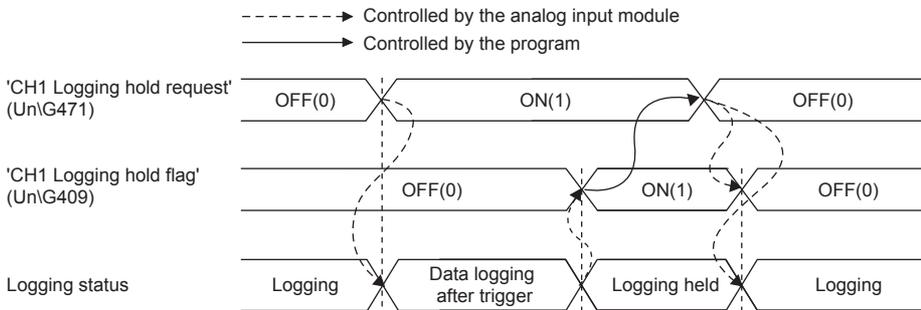
Logging does not stop when 'CH1 Logging hold request' (Un\G471) is changed on→off before ON (1) is stored in 'CH1 Logging hold flag' (Un\G409).
