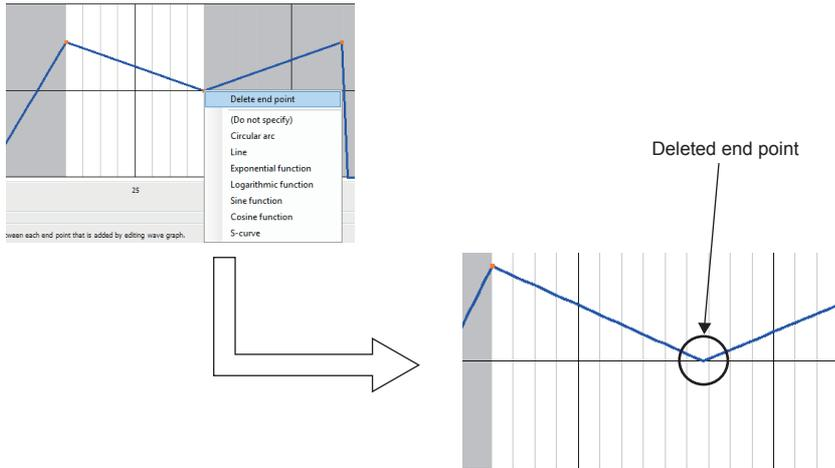
**4.** Set the wave between terminal points in the right-click menu or "Wave Specification" in "Wave Detail Setting".
