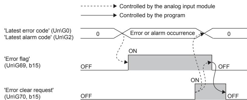
'Error flag' (Un\G69, b15), 'Latest error code' (Un\G0), and 'Latest alarm code' (Un\G2) are cleared at the timing when 'Error clear request' (Un\G70, b15) turns off→on.
