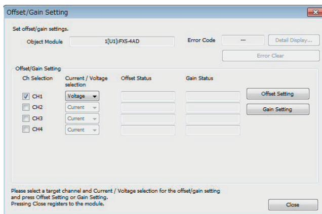
4. Mark the checkbox of the channel (CH1) where offset and gain values are to be set.
