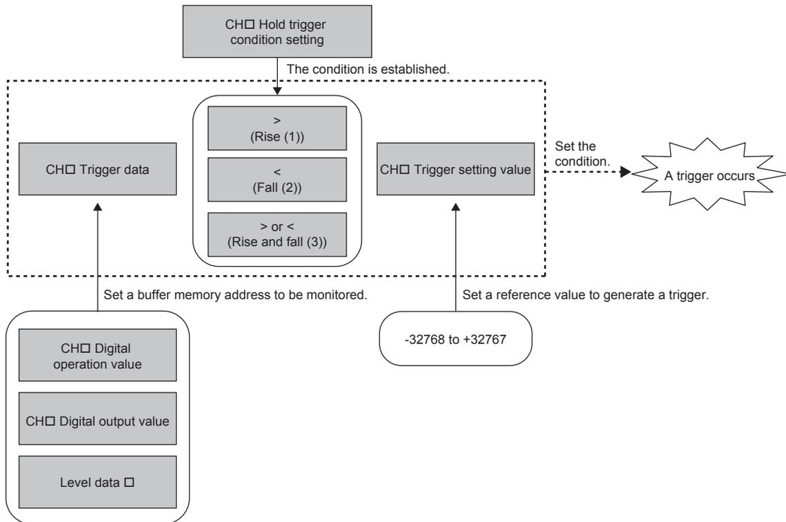
For example, to generate a hold trigger when a value in CH1 Digital output value exceeds 10000, set it as follows.
