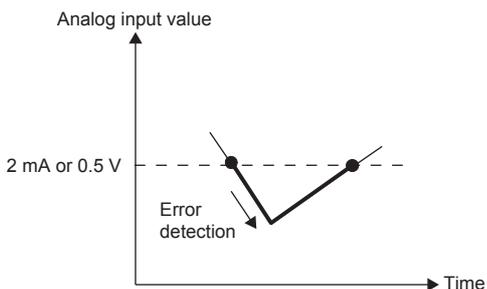
The settings for 'CH1 Input signal error detection lower limit setting value' (Un\G529) and 'CH1 Input signal error detection upper limit setting value' (Un\G530) are ignored.
