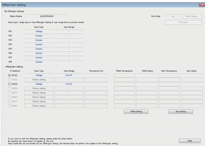
6. Input the offset value voltage "0 V" to the terminal of the target channel (CH1) and click the [Yes] button.
