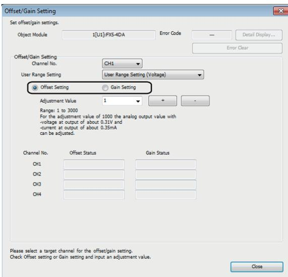
6. Select the adjustment amount of the offset or gain value from "1", "100", "500", "1000", "2000", and "3000". Alternatively, the adjustment amount can be set also by entering any numerical value from 1 to 3000.
