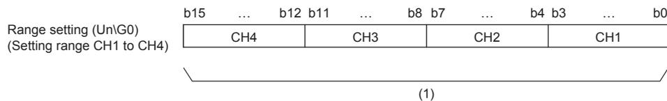
Set the following setting values for the bits corresponding to each CH.
