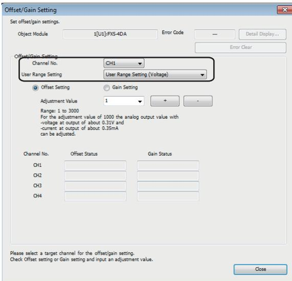
5. Specify the offset or gain setting using the radio button. (Perform step 6 and later only when the offset setting is specified in this step.)
