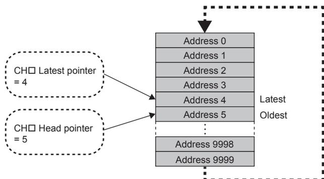
The head pointer does not change (fixed to 0) until CH1 Logging data (Un\G10000 to Un\G19999) becomes full after the logging start. (fixed to 0).
