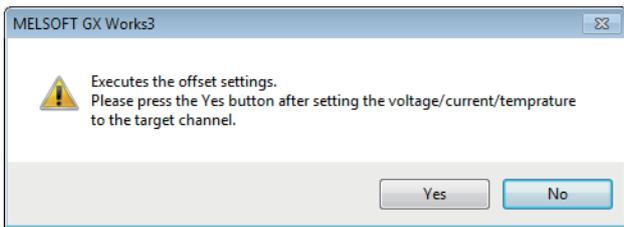
7. Input the offset value temperature "0°C" to the terminal of the target channel (CH1) and click the [Yes] button.
