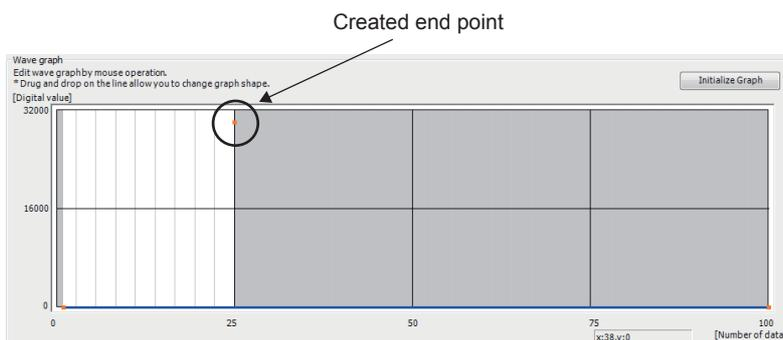
To delete it, move the mouse pointer to the terminal point and select "Delete End Point" from the right-click menu. Once the mouse pointer moves to the terminal point, its displayed shape changes to  $\oplus$ .
