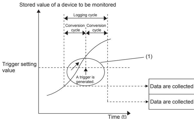
(1) The data at the timing when a trigger is generated is not stored in the buffer memory area.
