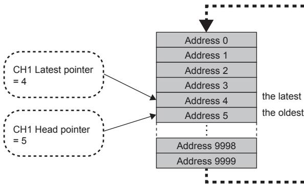
The head pointer does not change until CH1 Logging data (Un\G10000 to Un\G19999) becomes full after the logging start (fixed to 0).
