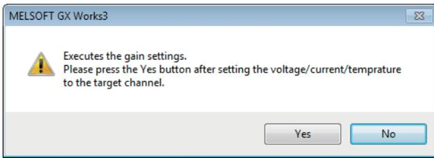
8. Input the Gain value voltage "5 V" to the terminal of the target channel (CH1) and click the [Yes] button.
