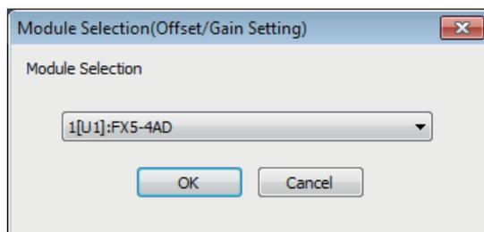
2. Select the target module for the offset/gain setting, and click the [OK] button.
