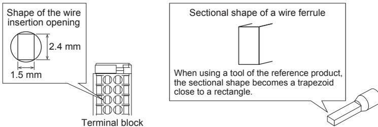
The following table shows wire ferrules and its associated tools compatible with the terminal block. The shape of the wire ferrule differs depending on the crimp tool to be used, use the reference product. If the product other than referenced products is used, the wire ferrule cannot be removed. Sufficiently confirm that the wire ferrule can be removed before use.
