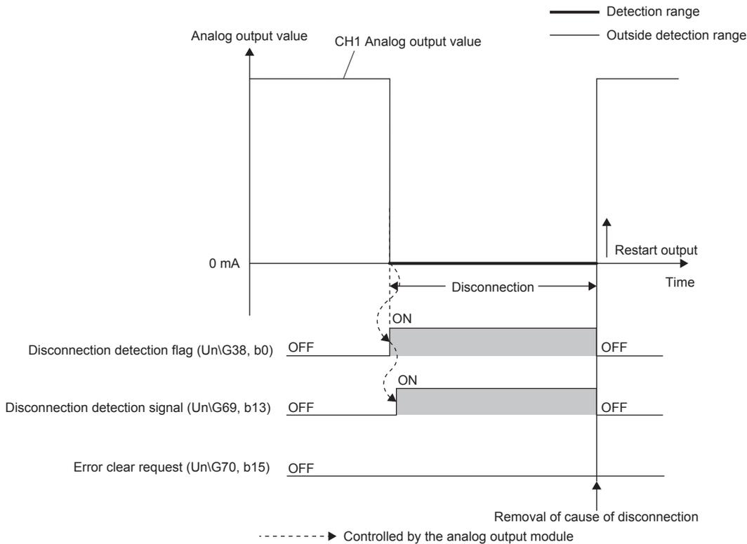
At the same time analog output restarts, the disconnection detection flag (Un\G38) of the corresponding channel is cleared. In addition, when the analog output of all channels restarts, 'Disconnection detection signal' (Un\G69, b13) is cleared.
