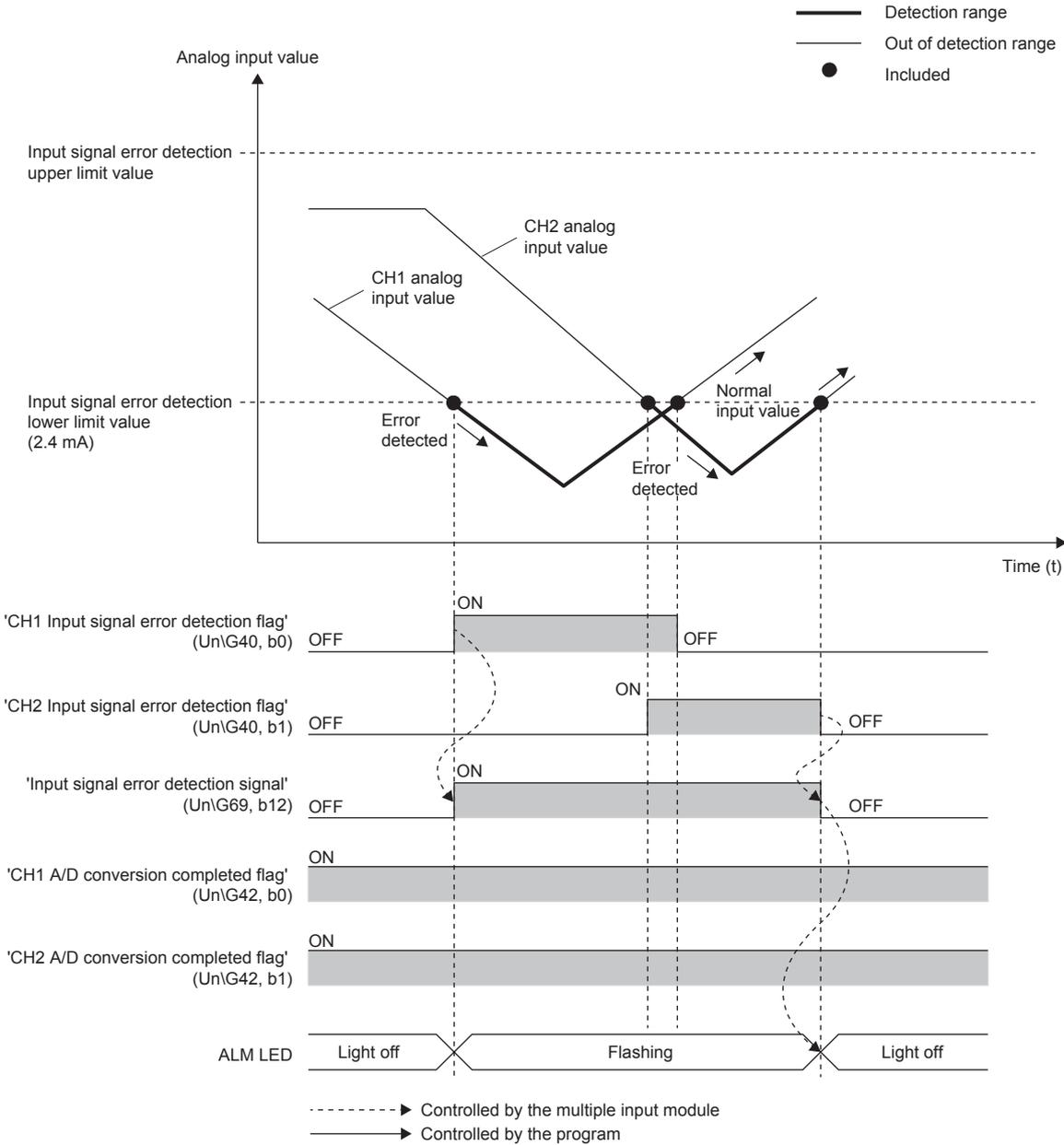
**■When Input signal error auto-clear enable/disable setting is set to Disable (1)**
