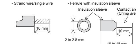
Check the shape of the wire insertion opening with the following chart, and use the smaller wire ferrule than the described size. Also, insert the wire with care so that the wire ferrule is in proper orientation. Failure to do so may cause the bite of the terminal and the damage of the terminal block.
