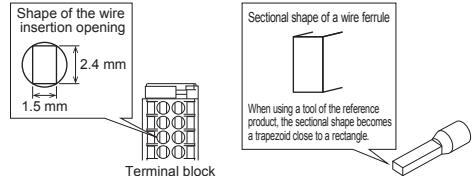
The following table shows wire ferrules and its associated tools compatible with the terminal block. The shape of the wire ferrule differs depending on the crimp tool to be used, use the reference product. If the product other than referenced products is used, the wire ferrule cannot be removed. Sufficiently confirm that the wire ferrule can be removed before use.
