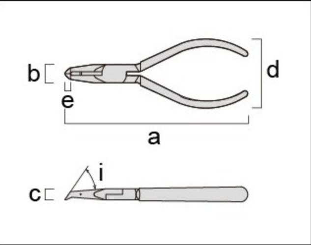
Most suitable to finish tunnel gate and pin gate
