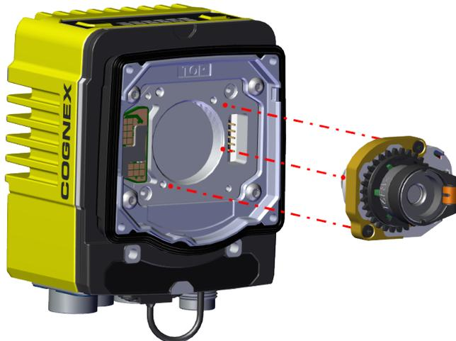
4. Screw in the four M3 x 6.35 screws from the illumination module into the reader.
