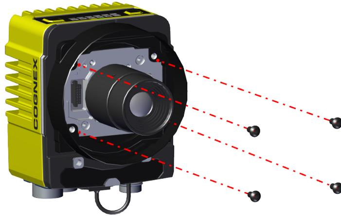
4. Push the lens cover onto the bayonet mount.
