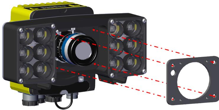
5. Place the lens cover over the lens. Tighten the M3x30 screws on the lens cover by using 50 Ncm.
