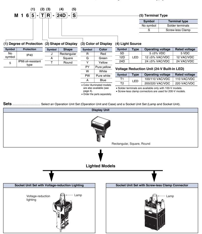
the Display, Case, Lamp, and Socket. Not all combinations are possible. Ask your OMRON representative for details.
