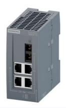
SCALANCE XB004-1G unmanaged Industrial Ethernet Switch for 10/100/1000 Mbit/s; for setting up small star and line topologies; LED diagnostics, IP20, 24 V DC power supply, with 4x 10/100/1000 Mbit/s RJ45 ports electrical and 1 x 1000 Mbit/s SC-port optical (multimode, glass), up to max. 750 m Manual available as a download .
