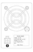
Connect Power Cable to 4Pin I/O connecter to supply DC24V to the product, and connect ground wire at the opposite end to the ground.
