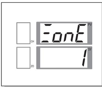
That is, whenever the
