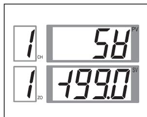
2. Press the **←/RS** key once and the first digit "9" of SV will flash. Press the **←/RS** key to move the digit, use the **↑/↓** key to set 300.0, and then press the **ENT** key to set.
