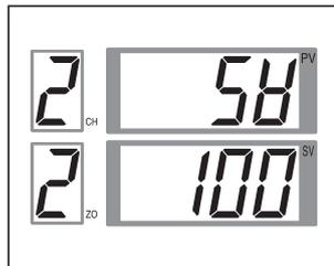
5. To change the zone number, press the
