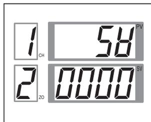
3. Press the CH key once to change the channel number from "1" to "2". This will change the channel number from "1" to "2".
