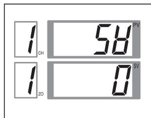
2. Each time press the
