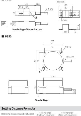
Detecting distance can be changed by the shape, size or material of the target.
