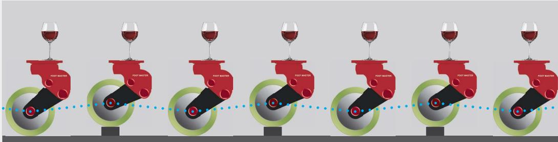
FOOT MASTER® shock absorbing casters using special rubber springs absorbing fine vibrations can not only protect products sensitive to shocks such as semiconductors and glass during movement, but can reduce even general natural noises as well as road-surface friction noises generated during the process of towing.
