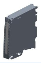
SIMATIC S7-1500 Analog input module AI 4xU/I/RTD/TC ST, 16 bit resolution, Accuracy 0.3%, 4 channels in groups of 4; 2 channels for RTD measurement; Common mode voltage 10 V; Diagnostics; Hardware interrupts; Delivery including push-in front connector, infeed element, shield bracket, and shield terminal
