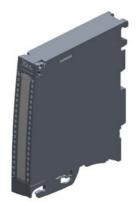
SIMATIC S7-1500, analog output module AQ 2x U/I ST, 16-bit resolution accuracy 0.3%. 2 channels in groups of 2, diagnostics; substitute value; the module supports the safety-oriented shutdown of load groups up to SIL2 according to EN IEC 62061:2021 and Category 2 / PL c according to EN ISO 13849-1:2015. delivery including front connector push-in, infeed element, shielding bracket and shield terminal
