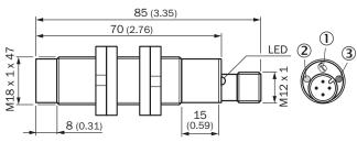
① Potentiometer for sensitivity adjustment
