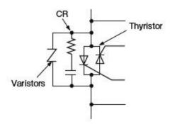
Varistors and C-R circuits are included so that surge voltage due to SSCswitching and lightening can besuppressed to protect the control andmain circuits.
