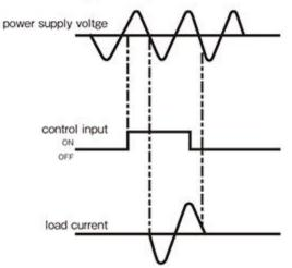
The SSC is also available with a zero-cross switching function to enable load current switching at the point where the line voltage is near zero to suppress excessive inrush current in the load circuit.
