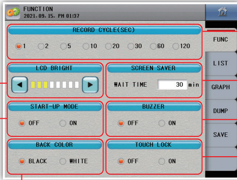
Fig. 31) Operating configuration screen
